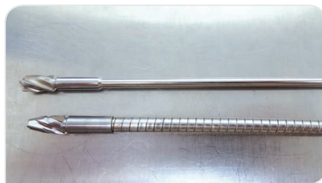
Figure 1. Semi-rigid intramedullary orthopedic reamer (above) and flexible intramedullary reamer for humerus used as a sample in this study (below).
