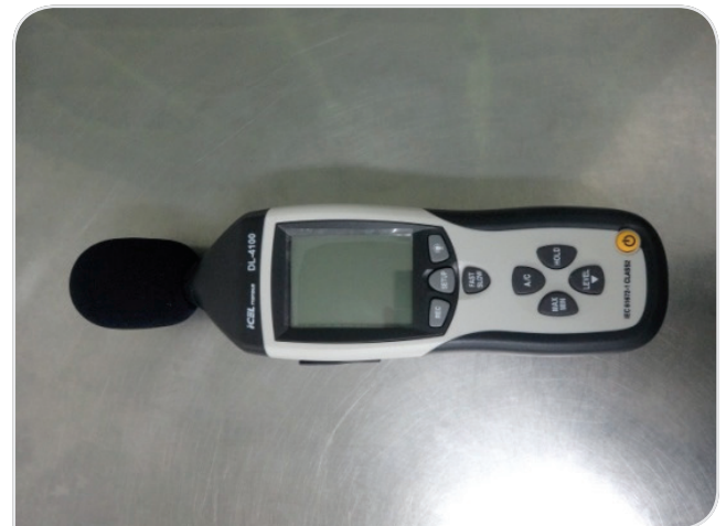
Figure 3. Sound meter Icel Manaus DL-4100 ® , device was used for measuring. Personal collection. São José dos Campos (SP), Brazil, 2014.
